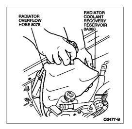
5. Remove the radiator coolant recovery reservoir.
