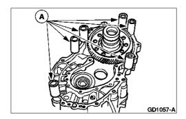
4. Set the transaxle case on the converter housing, then install the six collar bolts and washers (part of T88C-77000-JF).
