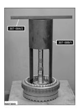
18. Using a press, compress the overdrive clutch piston return spring and install the snap ring.
