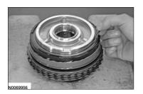
19. Remove and discard the direct clutch piston.
