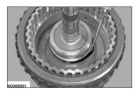
14. Remove and discard the overdrive clutch piston outer seals from the piston.
