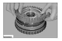
18. Remove the rear direct clutch piston seal.
