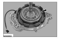
13. Remove and discard the overdrive clutch piston inner seal.
