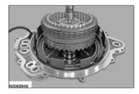
11. Apply air pressure to the overdrive piston port on the rear cover and remove the overdrive piston.
