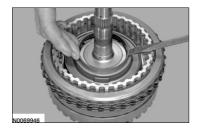
9. Remove the overdrive piston return spring.
