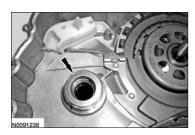
82. Simultaneously install the drive/driven sprocket and chain assembly. Lightly tap on the driven sprocket to be sure it is fully seated in the case.
