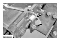
77. Install the 5 new clutch feed seals.
