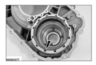
96. Seat the snap ring using a suitable tool.
