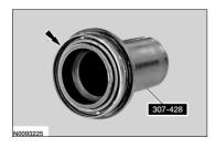
93. Using the RH Halfshaft Fluid Seal Installer 307-428, install the new RH halfshaft seal.
