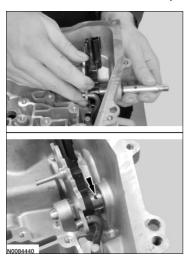
75. Install the manual control shaft roll pin.
