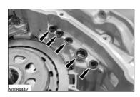
78. Position the transmission fluid baffle in place.
