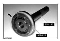
91. Using the Handle 205-153 and Differential Seal Installer 307-626, install the new RH halfshaft seal.
