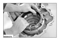
95. *NOTICE:* Be sure the flat side of the beveled snap ring is facing down or the ring can come loose, causing damage to the transaxle.
