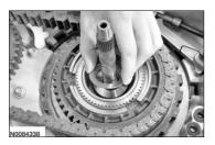
84. Install the No. 13 thrust washer.
