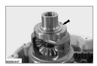
88. Install the Turbine Shaft Seal Protector 307-635 on the input shaft.
