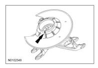
3. Cut the brake disc shield and remove it from the wheel knuckle.
