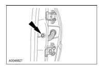
2. Align the door latch striker to specifications. For additional information on door clearances, refer to <u>Section 501-35</u>.
