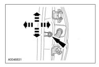
3. Tighten the door latch striker to 40 Nm (30 lb-ft).
