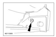
9. Remove the six torx screws from the refrigerator.
