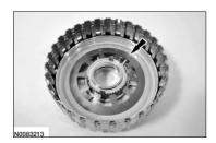
10. Install the forward clutch on the front pump to remove the forward clutch piston. Apply a small amount of shop air to remove the piston.
