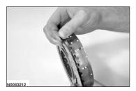
9. Remove the forward clutch return spring.
