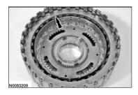
5. For correct alignment during assembly, make an identifying mark on the balance dam and the center part of the housing.
