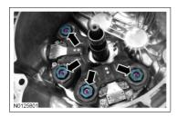
5. Install clutch actuator lever locks as shown if available.
