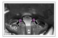
6. NOTICE: Be sure to properly handle the actuator lever as shown or damage may occur.
