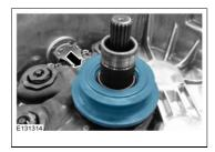
13. Install the clutch. For additional information, refer to <u>Clutch</u> in this section.
