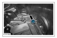
3. NOTICE: Be sure to properly handle the actuator lever as shown or damage may occur.
