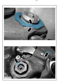
10. Remove the clutch actuator lever locks if installed.
