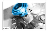
4. NOTICE: Remove the spring retainer bolts by loosening them slightly in an alternating pattern or damage can occur to the clutch actuator levers.
