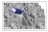
3. **NOTE:** The number on the valve tappet reflects the thickness of the valve tappet. For example, a tappet with the number 3.310 has the thickness of 3.31 mm (0.13 in).
