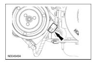
14. Position the lower radiator hose assembly into the vehicle.Connect the lower radiator hose to the radiator.
