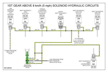
In 2nd gear, the forward (1, 2, 3, 4) clutch remains applied. SSC applies varying pressure to the 26 regulator and latch valves through the VBS CB26 hydraulic circuit to apply the intermediate (2, 6) clutch.
