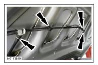
60. Install the 2 windshield washer hose retainers and the 8 hood insulation pin-type retainers (2 shown).
