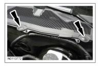
56. **NOTE:** The engine appearance cover rubber grommets may remain on the cover. If so, remove the grommets from the cover and install them on the intake manifold before installing the cover.
