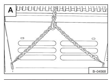
Use a punch and hammer, remove both hinge pins **[B]**. Lift the door from the loader frame.
