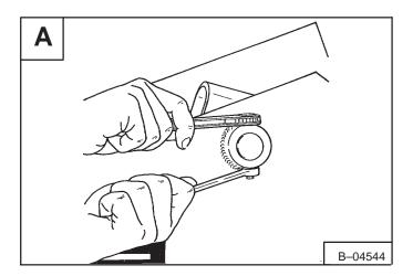
Use a punch and soft hammer, remove the pivot pin at the lift arm (both sides) **[B]**
