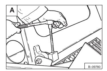
Remove the retainer clip at the upper pivot pin  $\ensuremath{\left[ B\right] }$  .
