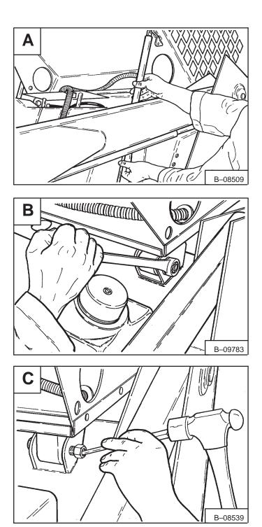
Remove the nuts from the pivot bolts [B].
