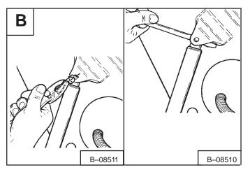
Remove the retainer clip at the lower pivot pin  $\circ{[C]}$ .
