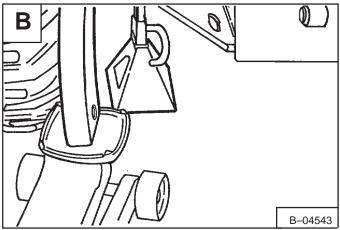
Remove the lock nut and bolt  $\c[C]$ .
