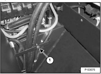
Loosen the mounting bracket bolt (Item 1) [Figure 50-10-12].
