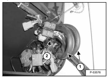
Remove the two A/C hoses (Item 1) and harness (Item 2) [Figure 50-10-13] completely from the rear corner of the cab.
