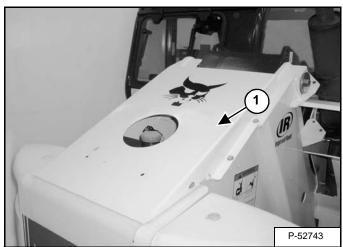
Remove the rear cover (Item 1) [Figure 50-10-22] from the machine.
