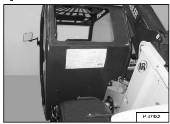
Lift and remove the operator cab [Figure 50-10-27].
