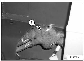
Temporarily remove the protective covering (Item 1) **[Figure 50-10-9]** from the A/C hoses and expansion valve.
