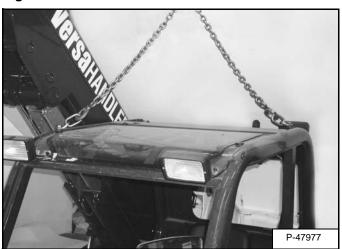
Install a hoist to lift and support the operator cab [Figure 50-10-20].
