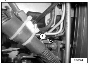
Remove the engine speed control cable (Item 1) [Figure 50-10-19] from the bracket.
