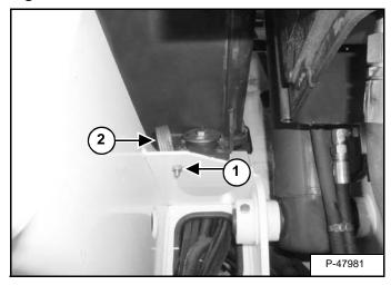
Remove the nut (Item 1) and bolt. Remove the grounding strap (Item 2) [Figure 50-10-23].
