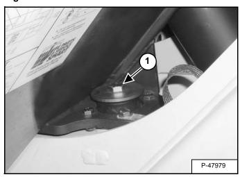
Loosen the rear mounting bolt (Item 1) [Figure 50-10-24], remove the nut.
