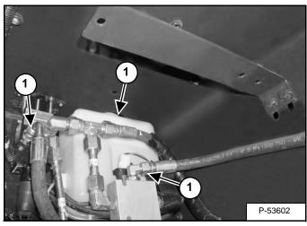
Remove the three hoses (Item 1) **[Figure 50-10-16]** from the brake valve. Remove any necessary tie straps.
