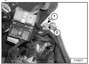
Remove the nut and washer (Item 1) and remove the ground wires (Item 2) [Figure 50-10-14].
