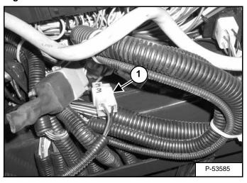
Unplug the connector (Item 1) [Figure 50-10-11] located under the fuse box.
