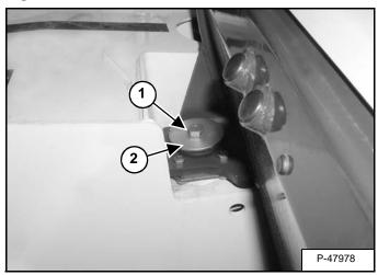
Remove the operator cab mount bolt (Item 1) and washer (Item 2) **[Figure 50-10-21]** from the front of the cab.
