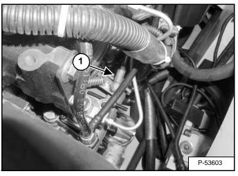
Remove the engine speed control cable (Item 1) [Figure 50-10-18].
