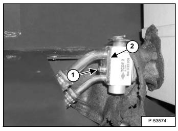
Remove the bolt (Item 1) and plate (Item 2) [Figure 50-10-10]. Remove the A/C hoses.
