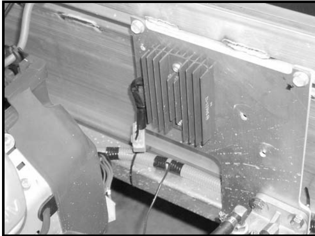
Figure 12a-4 Voltage Regulator
