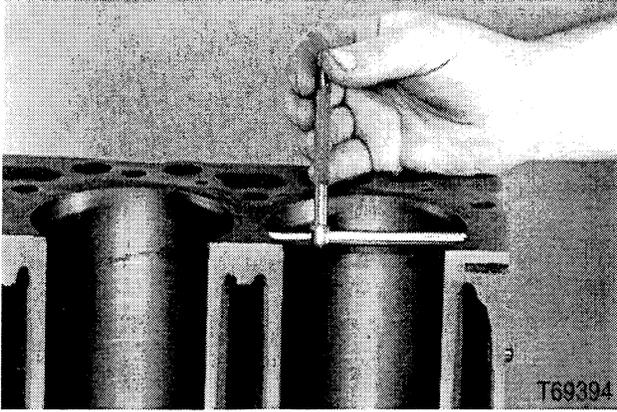
For 0.5 mm oversize pistons, machine cylinder bores to 102.40 to 102.44 mm.
