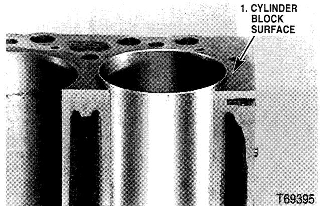
Cut the top of the sleeve flush to 0.025 mm above the cylinder block surface.
