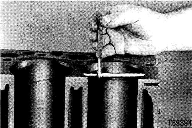
Bore each cylinder to a diameter of 104.485 to 104.515 mm down to the mark. Boring must be done in four steps with the final step taking a maximum of 0.125 mm. Let the block cool before the final step to prevent distortion.
