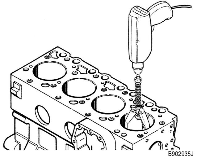
Use a cylinder hone and hone the cylinder bores to the following specifications. Use a lubricant/coolant with the hone to keep the stones clean and cool.
