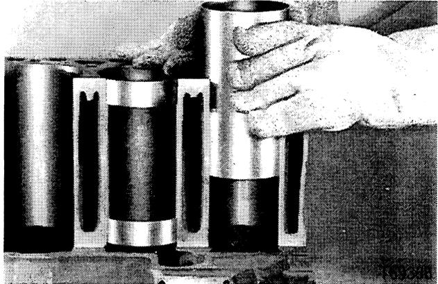
Freeze the sleeves at -12° C for at least one hour. Push the sleeves into the bore until the sleeve contacts the ridge at the bottom of the bore.
