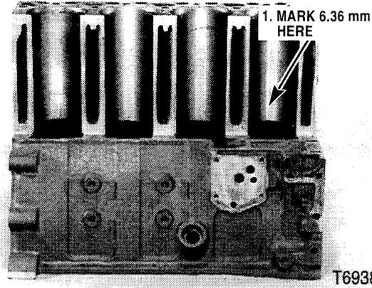
Put a mark on the cylinder bores 6.36 mm up from the bottom.
