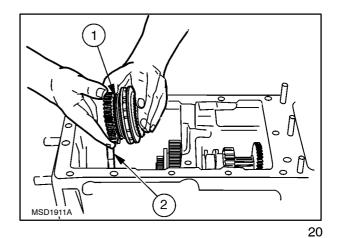
13. Remove the snap ring (1), extract the PTO gear unit (2) and recover the washer and bearing.
