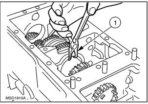
12. Move back the upper shaft, recover the synchroniser (1) on the 3<sup>rd</sup> and 4<sup>th</sup> gear and the engagement fork (2) on the 1<sup>st</sup> and 2<sup>nd</sup> gear.
