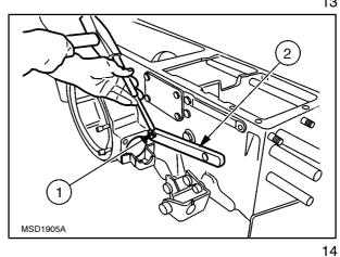
7. Unscrew the caps (1) and recover the springs and the check balls from the rods.
