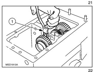
15. Extract the rear part of the main shaft (1) and recover the components (2).
