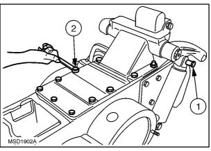
4. Using the hoist chains (1) raise the lift cover (2) and remove.
