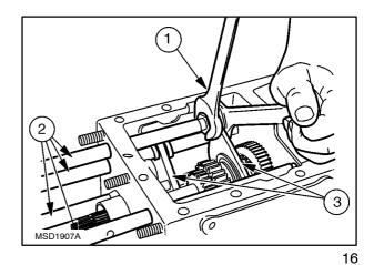
9. Remove the main shaft snap ring (1), remove the lubrication collar (2) and recover the spacer and the adjustment shims.
