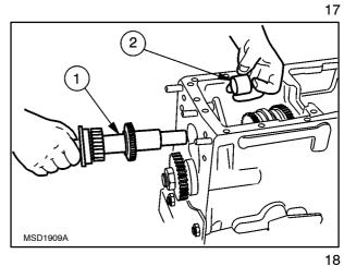
11. Remove the retaining snap ring (1) on the upper shaft.
