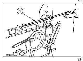
6. Extract the spring pin (1) to remove the creeper engagement lever (2).
