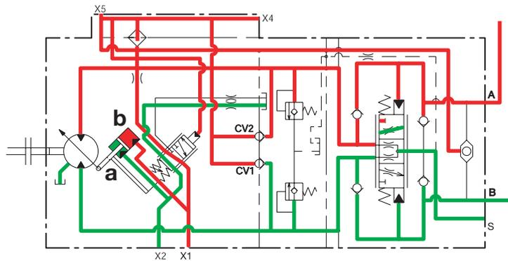
Fig 2. Operation at high pressure - 220bar
