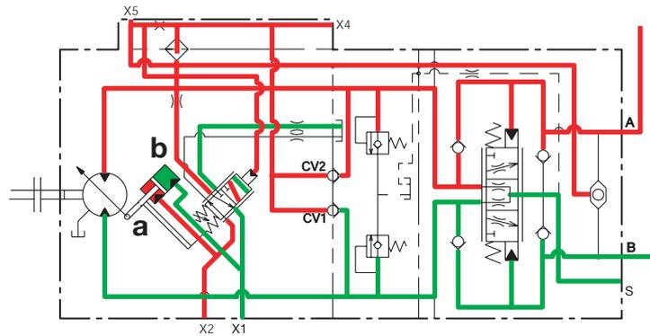
Fig 1. Operation below 210bar
