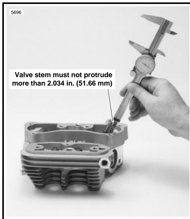
Figure 3-22. Measuring Valve Stem Protrusion
