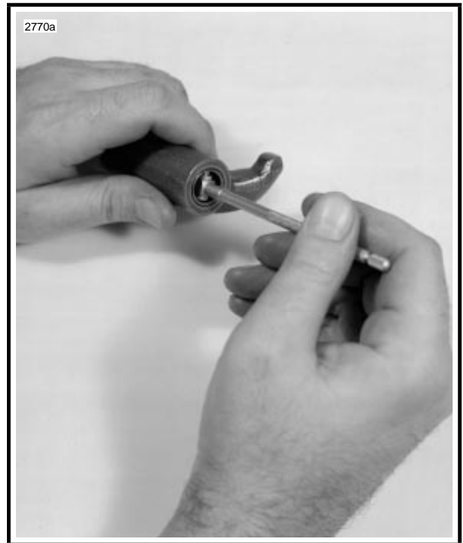
Figure 3-15. Measuring Rocker Arm Bushing Inner Diameter
