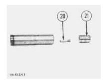
**16.** Remove pistons (20) and (21) from the servo valve cartridge.
