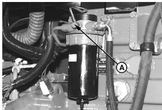
A—Air Bleed Valve
