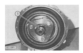
1. Use tool (A) to remove snap ring (1) from the shaft
