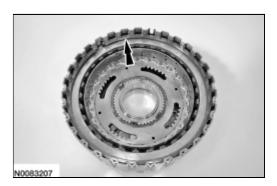
4. NOTE: Inspect the forward clutch drum and the friction and steel plates for damage. Install new
