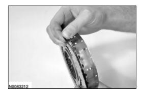
$9. \quad \hbox{Remove the forward clutch return spring}.$
