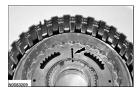
6. **NOTE:** The bottom of the Clutch Spring Compressor will need to be installed from the back side of the forward clutch assembly.
