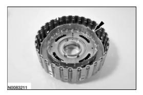
8. Remove and discard the O-ring seal from the balance dam.
