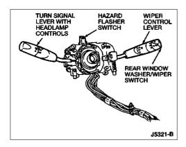
The windshield wipers are controlled by the wiper control lever, which is integral with the multi-function switch. The wiper control lever is located on the right side of the multi-function switch. To operate the windshield wipers, the ignition switch (11572) must be in the ACC or ON position. The windshield wipers have three fixed positions: OFF, LO and HI.
