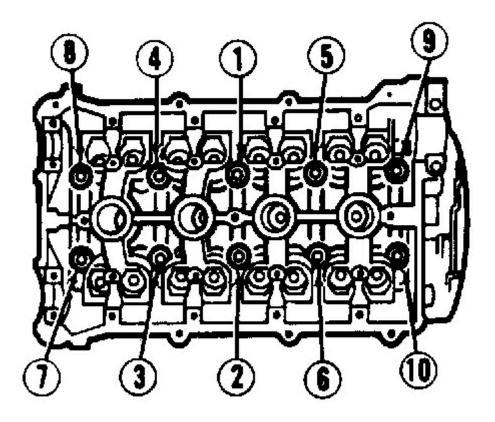
Fig. 2: Installing Cylinder Head Bolts (1.6L) Courtesy of FORD MOTOR CO.
