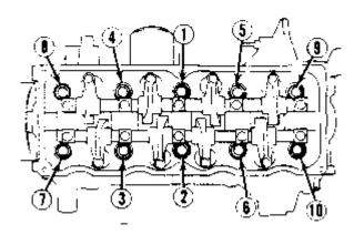
Fig. 1: Installing Cylinder Head Bolts (1.3L) Courtesy of FORD MOTOR CO.
