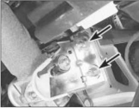
7.8 Two of the three nuts (arrowed) which secure the column height adjuster
