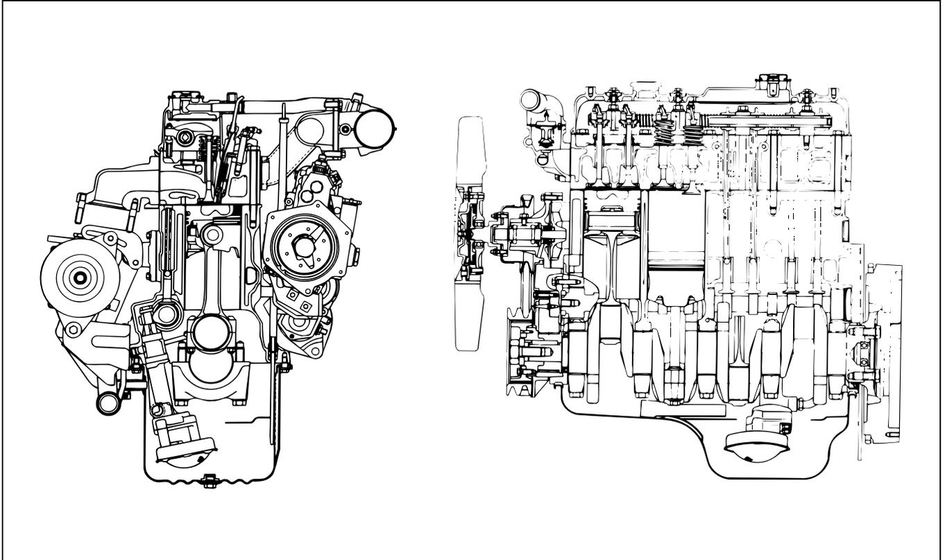
The A-4J Series of industrial engines features the unique ISUZU troidal square combustion chamber. This design provides superior fuel economy for a wide range.
