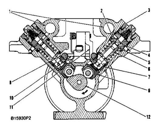
Cross Section Of The Fuel Injection Pump Housing
