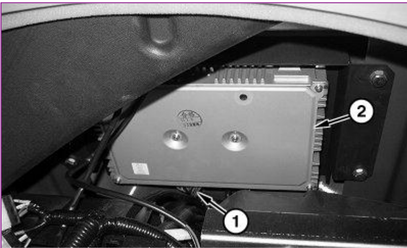
TX1003378A-UN: Main Controller
