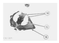
**10.** Remove metal gasket (16), and two journal bearings (14) from the rear side of the front cover assembly. Check the condition of two pins (15). If they are worn or damaged, replace them.
