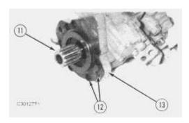
**NOTE:** Spline coupling (11) may have remained with the pump drive unit when the vibratory pump is removed.
