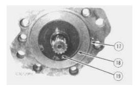
**NOTE:** It will be necessary to destroy seal (19) to remove it from the front cover assembly.
