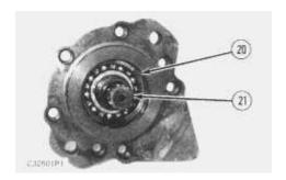
**12.** Remove snap ring (20) and pull shaft assembly (21) out of the front housing. This is a slip fit and therefore will not require the use of a press.
