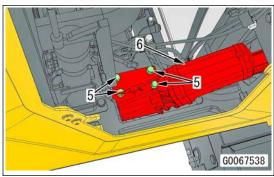
30. Loosen the nut (D5), and remove the installer (D).
