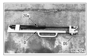
28. Install the gas spring (20a) with the pins (18) (2 pieces) and cotter pins (20) (2 pieces).
