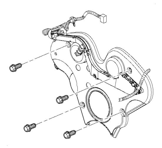
Fig. 328: Removing & Installing Front Timing Belt Cover Courtesy of GENERAL MOTORS CORP.
