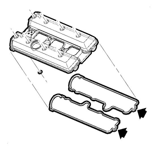
Fig. 329: Identifying Camshaft Cover Seals & O-Rings Courtesy of GENERAL MOTORS CORP.
