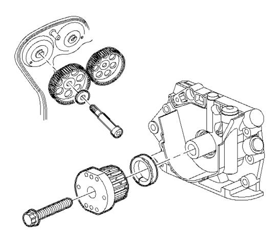
Fig. 332: Removing & Installing Camshaft Gear & Crankshaft Drive Gear Bolts Courtesy of GENERAL MOTORS CORP.
