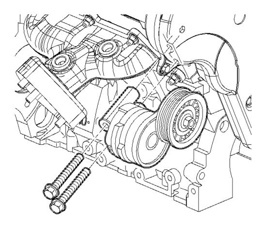
Fig. 326: Removing & Installing Drive Belt Tensioner Courtesy of GENERAL MOTORS CORP.
