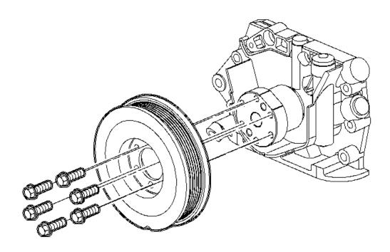
Fig. 327: Removing & Installing Crankshaft Balancer Courtesy of GENERAL MOTORS CORP.
