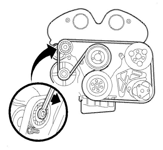
Fig. 325: Using 15 mm Wrench To Rotate Tensioner Pulley Courtesy of GENERAL MOTORS CORP.
