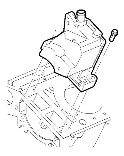
Fig. 324: Removing & Installing Engine Vent Housing Courtesy of GENERAL MOTORS CORP.
