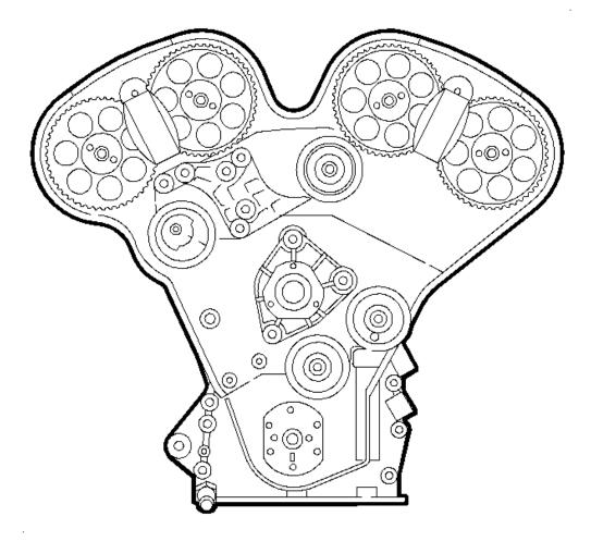
Fig. 331: View Of Installed Camshaft Locks Courtesy of GENERAL MOTORS CORP.
