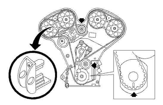
Fig. 330: Installation Of Special Tools For Camshaft Drive Sprocket Removal Courtesy of GENERAL MOTORS CORP.
