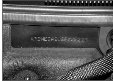
The chassis number is stamped on the bulkhead (passenger side) in engine compartment.
