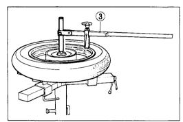
Attach the bead breaker 4 to the operation arm, and dismount the bead from the rim. Turn the wheel over and dismount the other bead from the rim.
