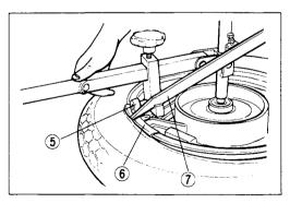
• Set the tire lever against the operation arm, and rotate the lever around the rim. Repeat this procedure to remove the other bead from the rim.
