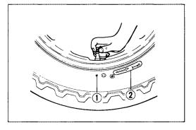
• Place the center shaft ① to the wheel, and fix the wheel with the rim holder ②.
