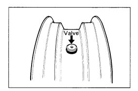
Inspect the removed valve core and replace with the new one if the seal rubber is abnormally deformed or worn.
