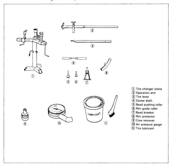
Remove the valve core from the valve stem, and deflate the tire completely.
