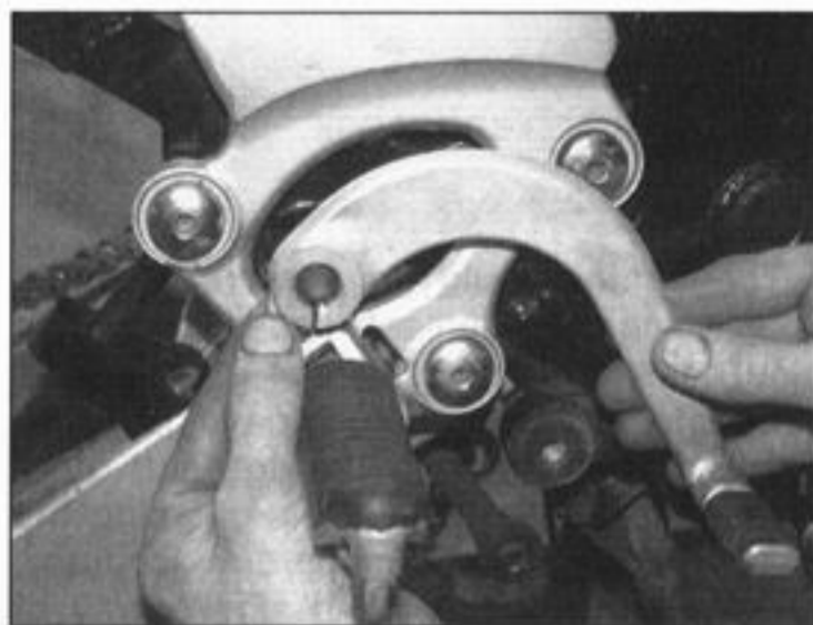
3.9b . . . then draw the pedal off the shaft . . .
