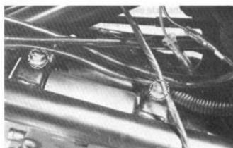
Remove the oil cooler joint hoses.
