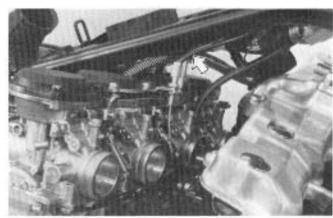
· Loosen and remove the exhaust pipe clamp bolts.
