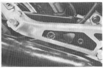
· Remove the ignition coils by loosening the nuts.
