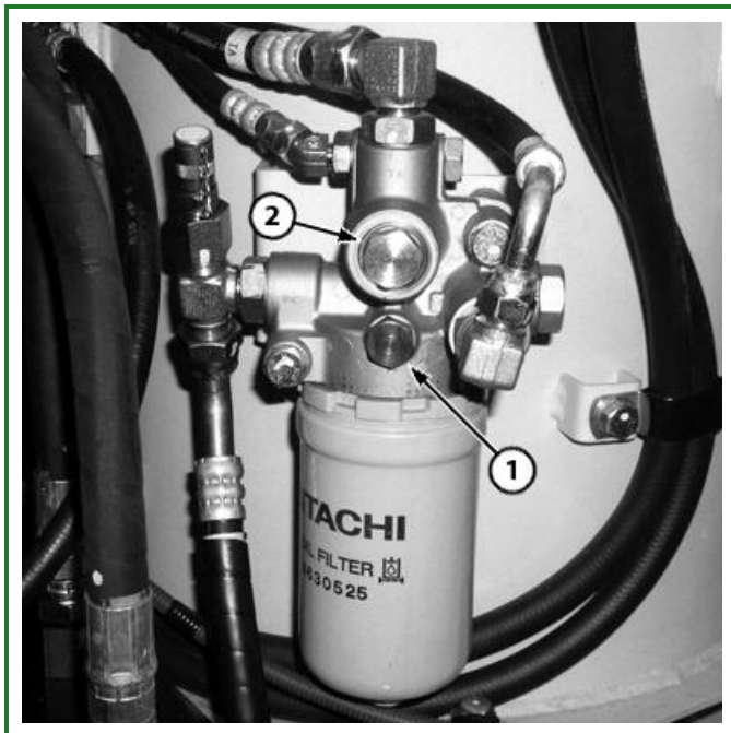
TX1034315A-UN: Pilot Pressure Regulating Valve and Test Port
