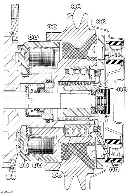
AA—Shaft Seal BB—Seal Seat CC—Pulley DD—Hub and Drive
