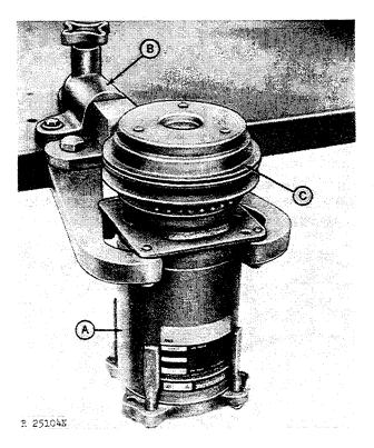
A-Compressor **B**—Bench Fixture C-Dust Cover
