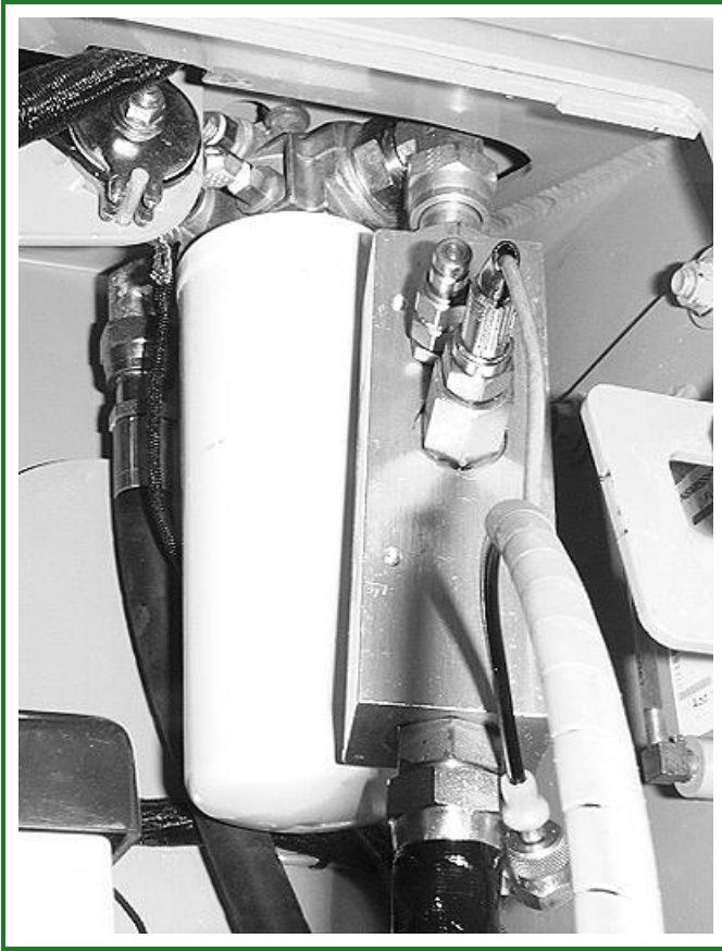
T116990B-UN: Flow Meter Shown Installed On Filter Inlet
