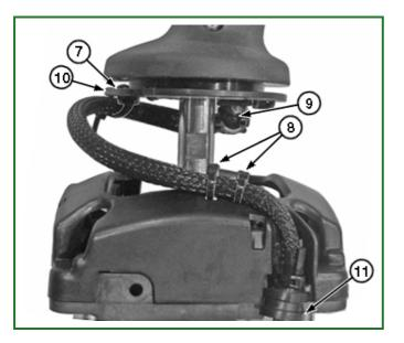
TX1128561A-UN: Joystick Harness Routing
