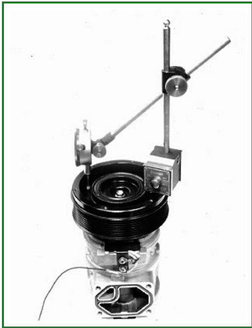
RW21159-UN: Clutch Hub Clearance
