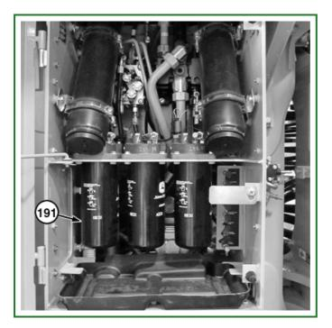
**TX1196771A-UN: Right Rear Axle Oil Filter** <u>LEGEND:</u> 191 - Right Rear Axle Oil Filter
