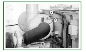
**T7134JJ-UN: Disconnect Wiring Leads** Disconnect wiring leads (A).
