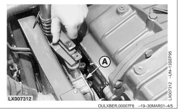
Disconnect transmission wiring harness ground connection and install JDG19 (A) lifting eye at range transmission using a cap screw.
