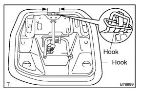
(c) Using a screwdriver, disengage the hooks and seat cushion cover together with the pad.
