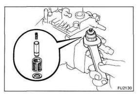
(d) Remove the fuel cut solenoid, O-ring, spring, valve, strainer and wave washer.
