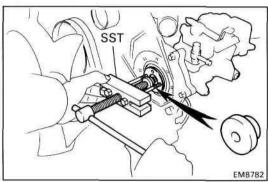
(c) Before removing the injection pump, check if the period lines are aligned.
