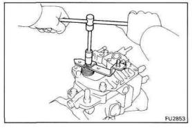
(b) Remove the nut, return spring guide, adjusting lever and return spring.
