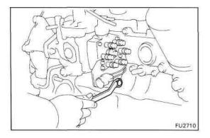
(b) Remove the bolt holding the injection pump to pump stay.
