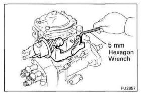
(c) Using a 5 mm hexagon wrench, remove the two bolts and PCS actuator assembly.
