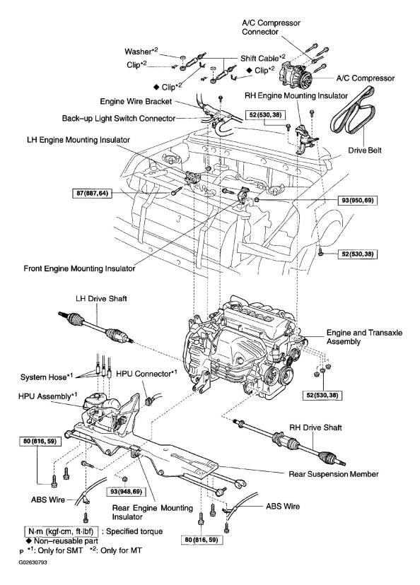
Fig. 172: Identifying Engine Unit Components (4 Of 5)
