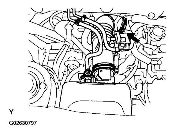
Fig. 176: Disconnecting Accelerator Cable Courtesy of TOYOTA MOTOR SALES, U.S.A., INC.
