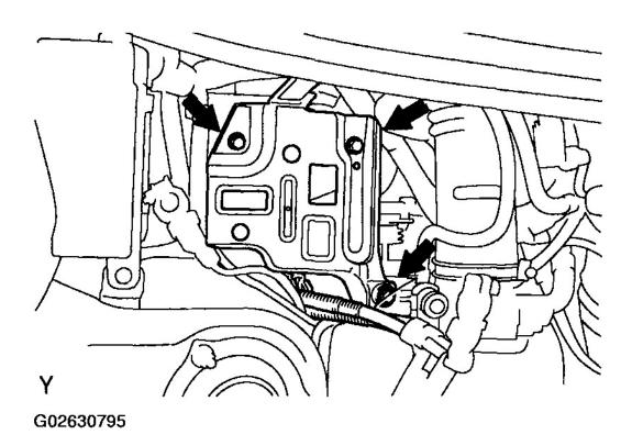
Fig. 174: Identifying Battery Bracket Bolts Courtesy of TOYOTA MOTOR SALES, U.S.A., INC.
