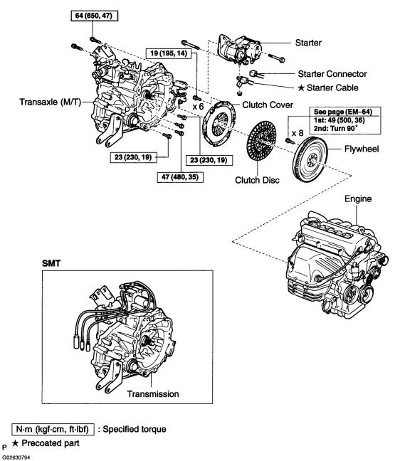
Fig. 173: Identifying Engine Unit Components (5 Of 5)
