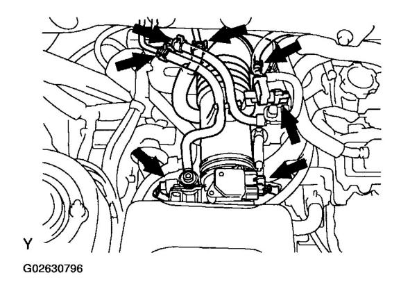
Fig. 175: Removing Intake Air Hose And Air Cleaner Cap Assembly Courtesy of TOYOTA MOTOR SALES, U.S.A., INC.
