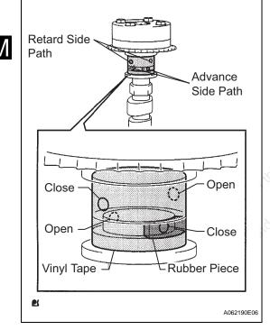
(f) When the camshaft timing gear comes to the most advanced position, release the air pressure of the timing retard side path, then release that of the timing advance side path. CAUTION:
